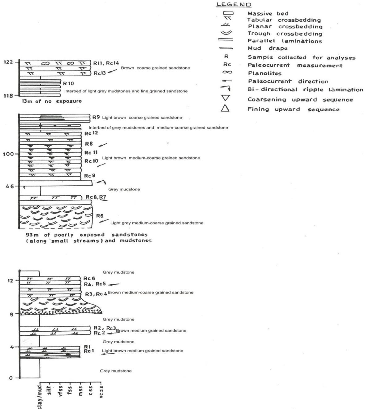
Fig.8 Section of Yolde Formation at Ruwan Kuka Village
