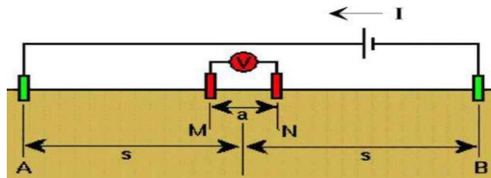
**Figure 2:** Schematic diagram of Schlumberger Configuration
