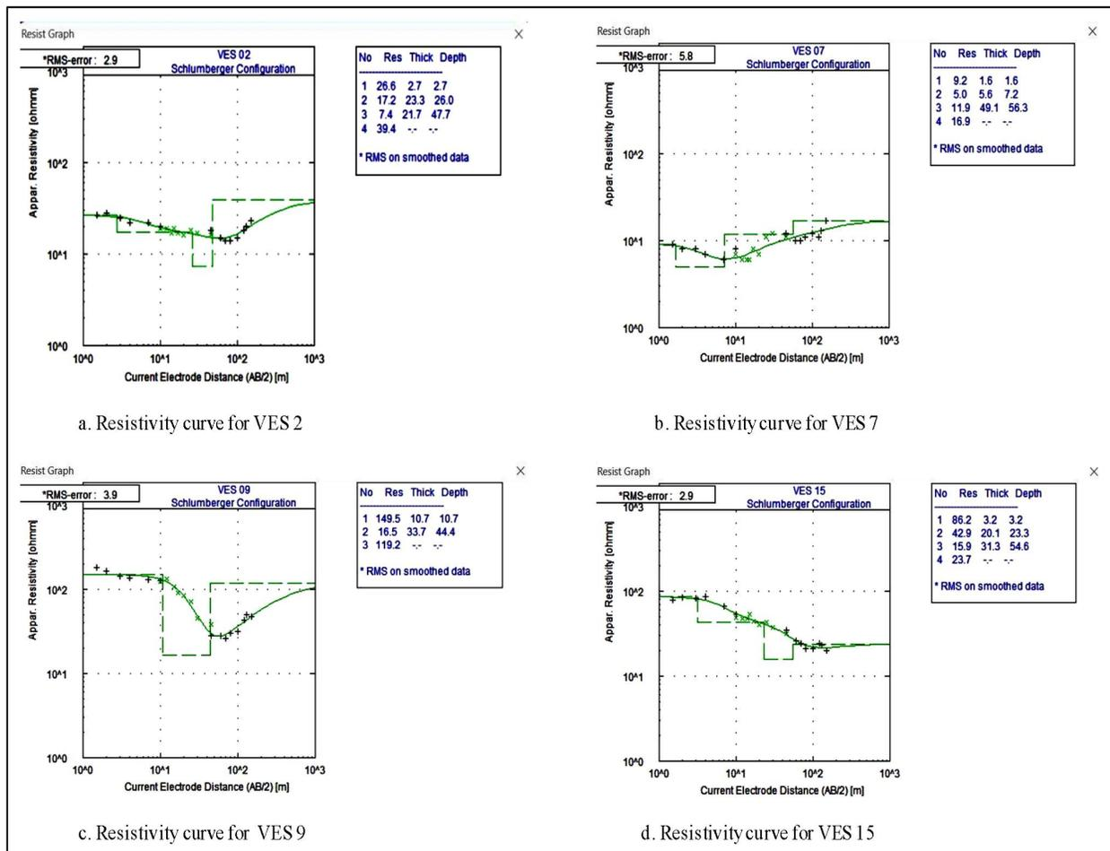
**Figure 3:** Resistivity curves for some selected VES locations
