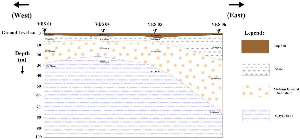
Figure 7: Geo-electric section along VES 01, 04, 05 and 06 plotted in an east- west direction.
