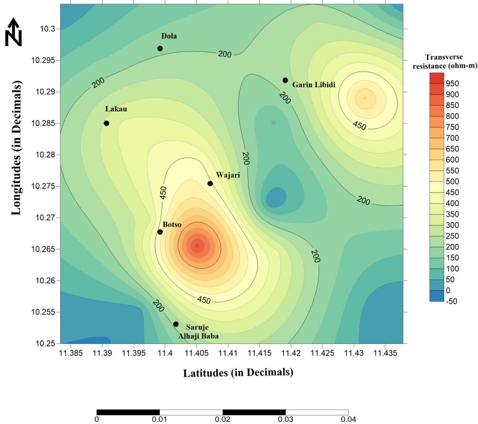
**Figure 12:** Transverse Unit Resistance Map of the study area (map scale is in Km).
