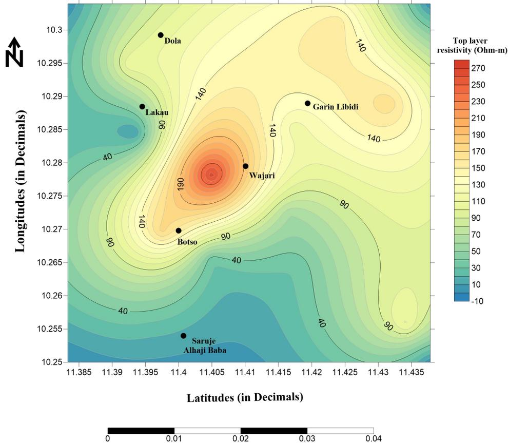
**Figure 10:** Top Soil/First stratum corrosivity map of the study area (map scale is in Km).
