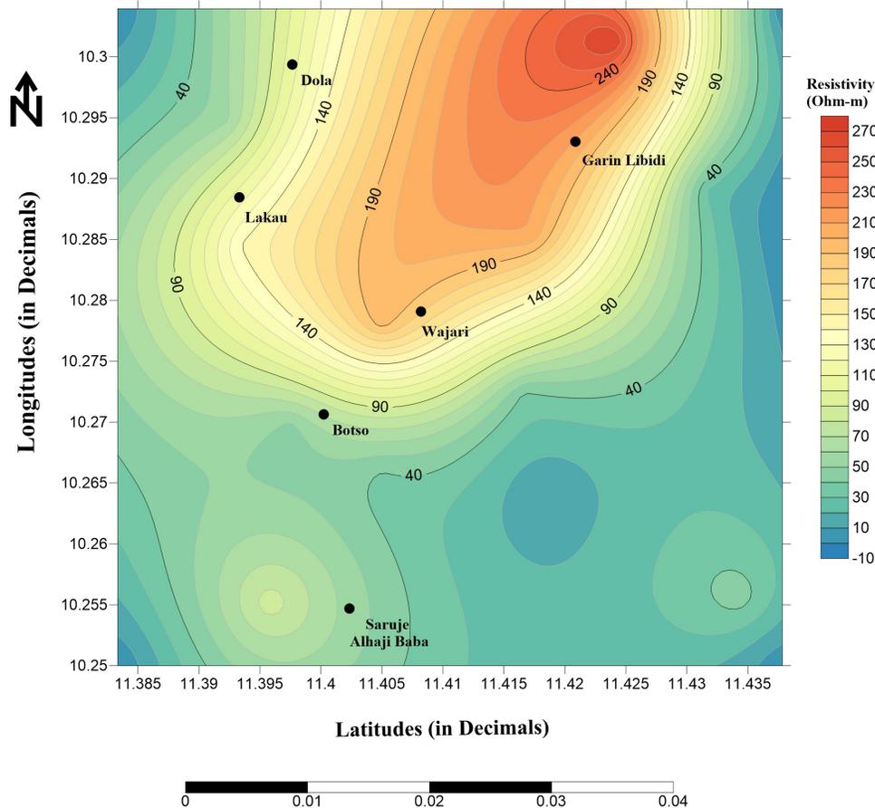
**Figure 9:** Iso-resistivity map of the study area at AB/2=30/2m (map scale is in Km).
