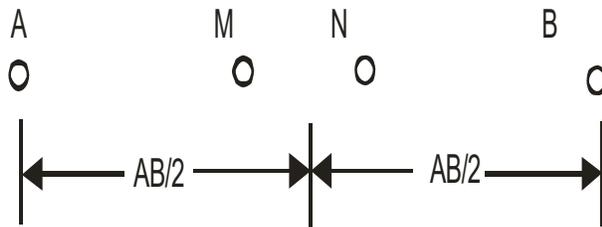
**Figure 3:** Schlumberger electrode arrangement showing position of electrodes.
