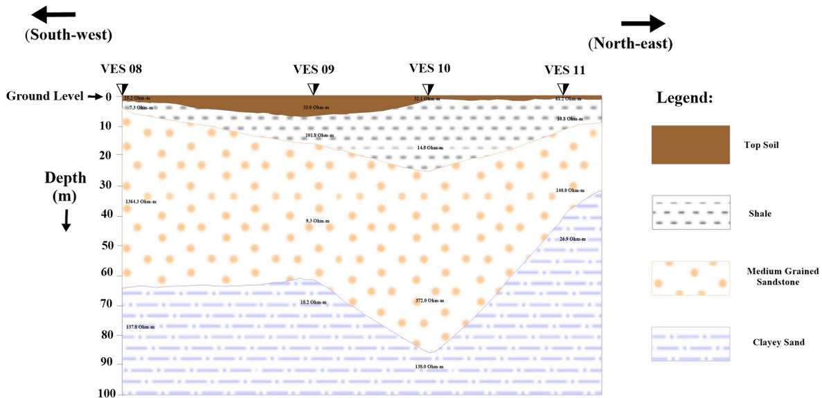
Figure 8: Geo-electric profile along VES 08, 09, 10 and 11 plotted in a northeast- southwest direction.
