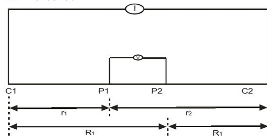
**Figure 4:** Schlumberger Electrodes Arrangement Showing Electrodes spread.
