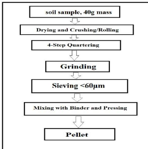
**Figure 1:** Sample Pelleting Prior to Analysis
