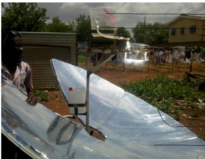
Figure 5: Experimental setup of parabolic dish concentrating system with thermal compensator.
