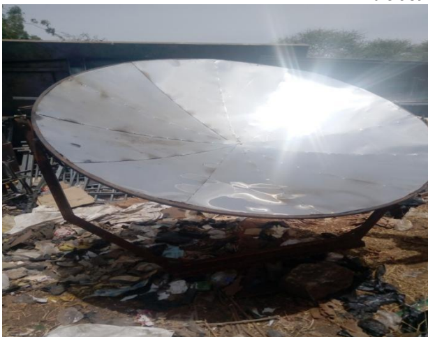
Figure 4: Constructed parabolic dish solar concentrating collector.
