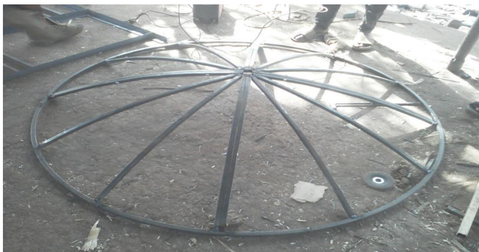
Figure 2: Assembled of trapezoidal petal shaped reflector of parabolic dish concentrator.
