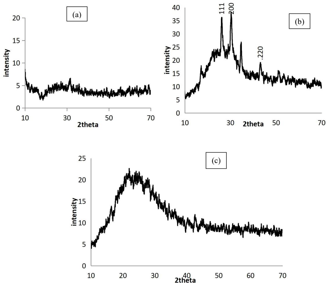
**Figure 1:** XRD patterns of PbS (a) deposited at 300° celcius, (b) annealed at 300°celcius and (c) annealed at 400°
