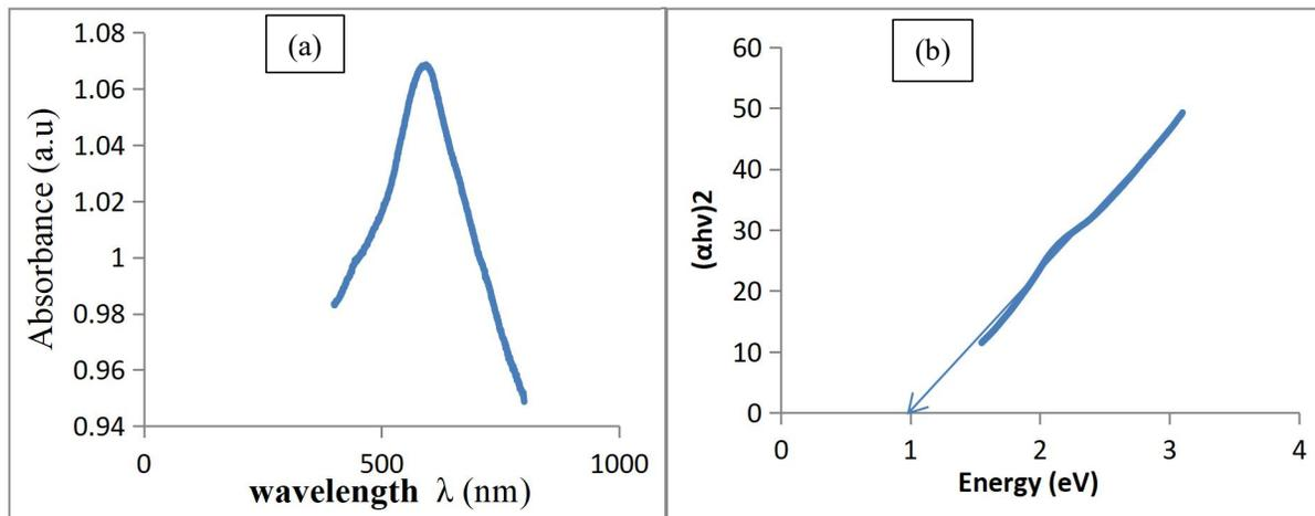
**Figure 3:** (a) Absorbance against Wavelength of PbS deposited at 300°C Thin Film and (b)  $(\alpha h\nu)^2$  against Energy of PbS deposited at 300°C Thin Film.
