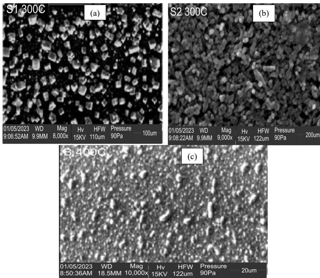
**Figure 2:** PbS films morphology (a) deposited at 300°C (b) annealed at 300°C and (c) annealed at 400°C.
