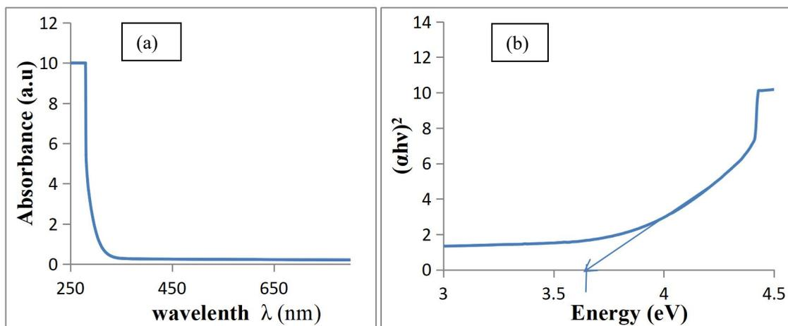
**Figure 4:** (a) Absorbance against Wavelength of PbS Thin annealed at Film 300°C and Figure 4(b)  $(\alpha h\nu)^2$  against Energy (eV) of PbS annealed at 300°C Thin Film.
