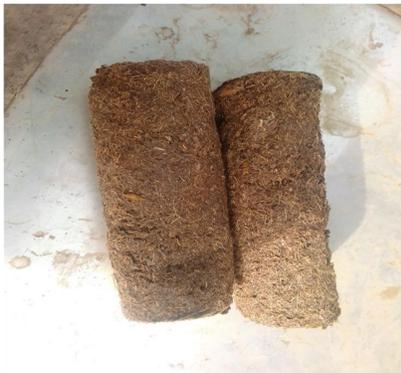
Figure 3: Palm Mesocarp Fiber Briquettes
