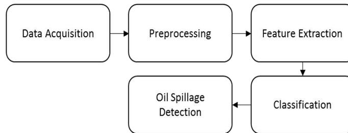
**Figure 1:** Block diagram of the proposed oil spill detection using neural network
