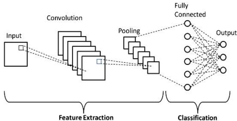
**Figure 2:** CNN architecture
