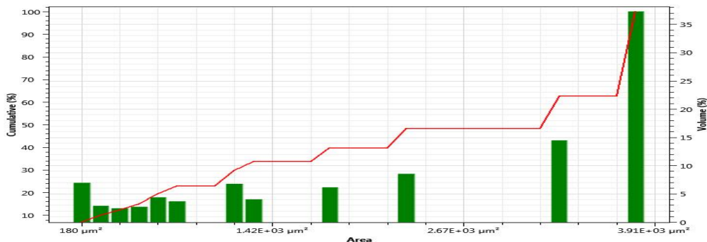
Figure 15. Graph of cumulative (%) against area of particles of catalyst produced by physical activation Cocos nucifera shell.
