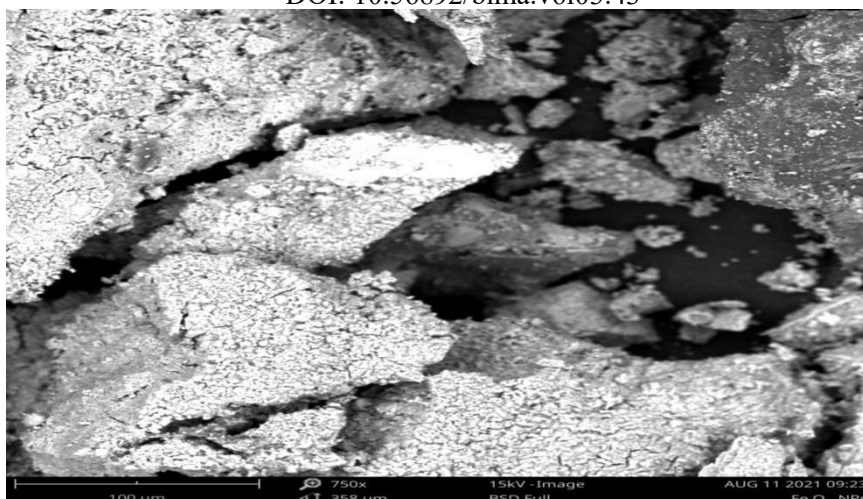
Figure 4: SEM micrographs of FeO NPs synthesized with Ziziphus M. extract
