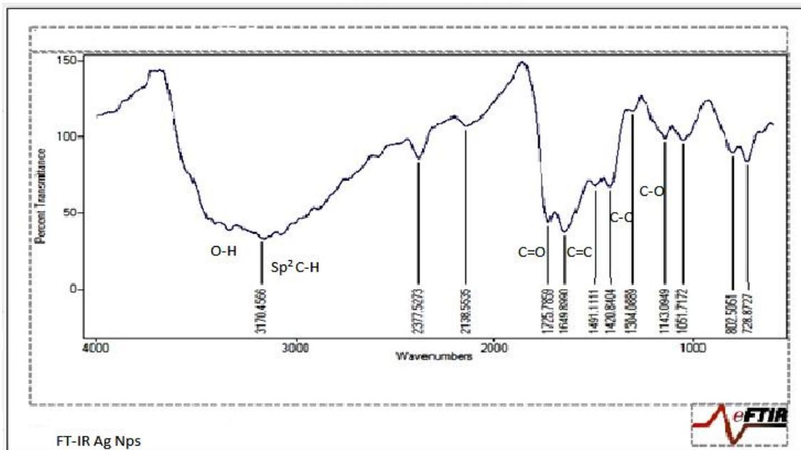
Figure 4: FTIR spectrum of synthesized silver nanoparticles using *Tagetes erecta* leaves
