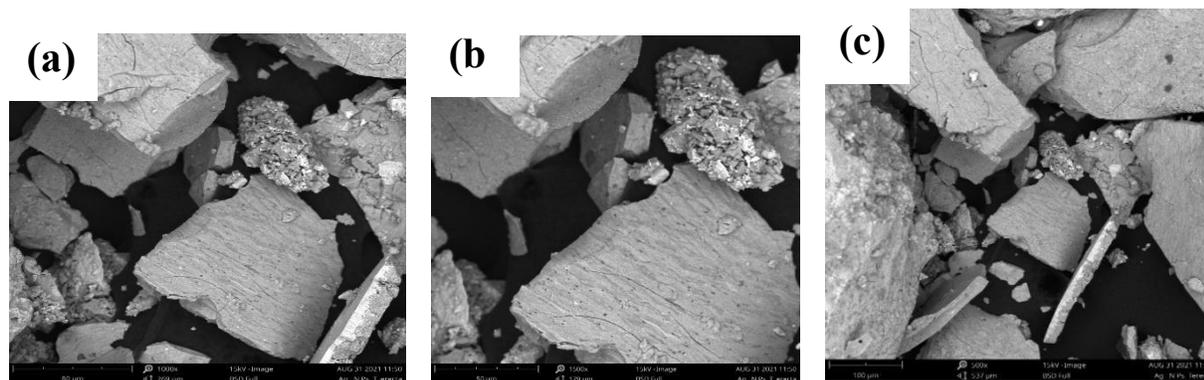
Figure 5: SEM image of synthesized AgNPs (a) 50 μm, (b) 80 μm and (c) 100 μm
