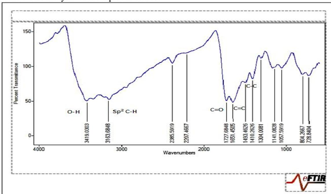
**Figure 3:** FTIR spectrum of aqueous extract of *Tagetes erecta* leave
