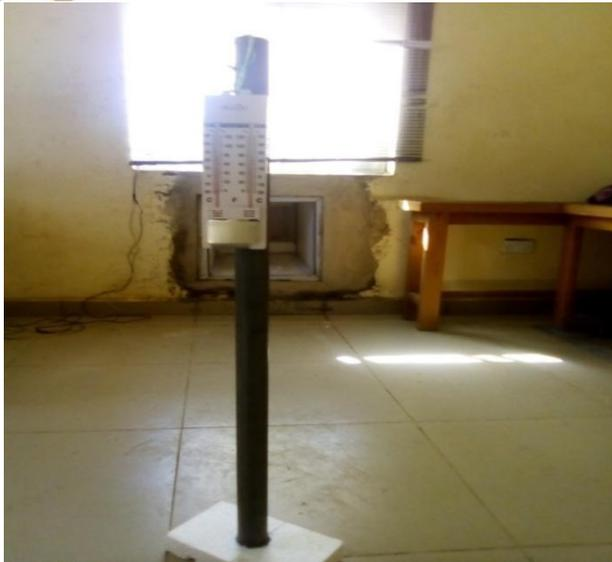
**Figure 2:** Hygrometer at the centre of office room at 1.1m above floor level
