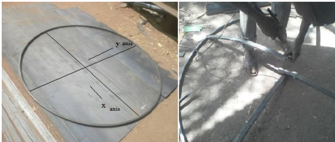
Figure 2: (a) Plate 1, Measuring parabolic dish geometry
