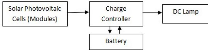
**Figure 1:** Block Diagram of Solar Street Lighting System using DC Lamp
