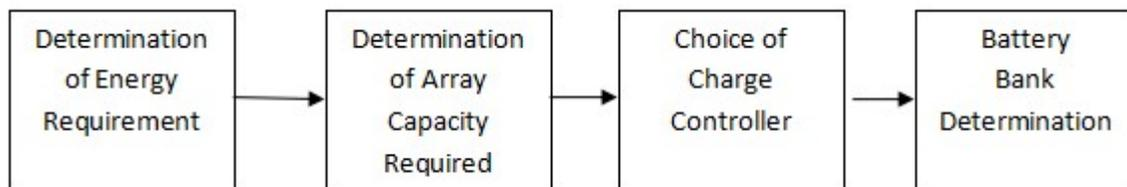
**Figure 2:** Block Diagram Summarizing the Method Used
