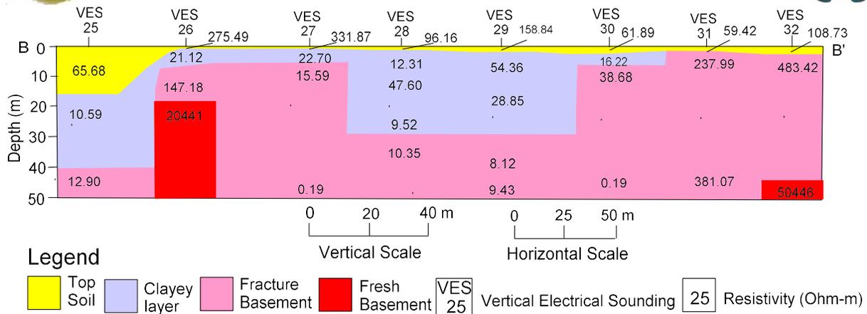
**Figure 11b:** 2-D Geoelectric sections along profile BB' of the study area northeastern Nigeria.
