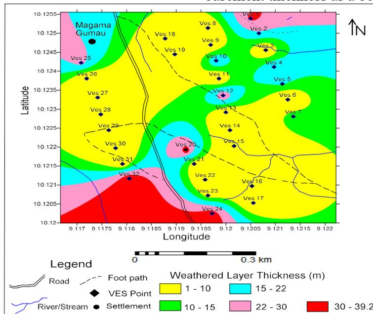
**Figure 5:** Weathered layer thickness map of the study area northeastern Nigeria.
