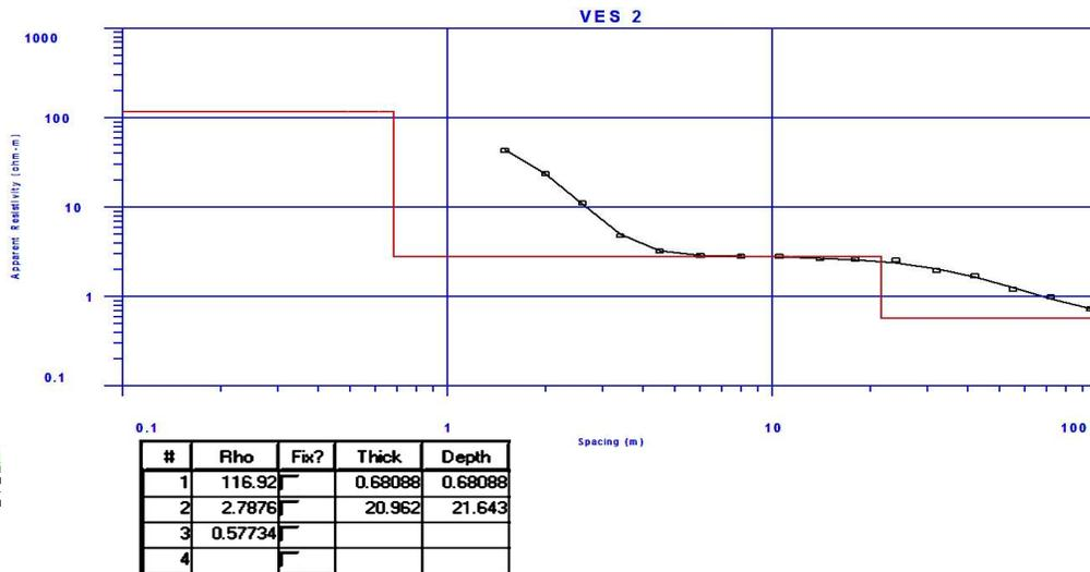
**Figure 3a:** Typical Q-type curve for 3 layered earth model of the study area northeastern Nigeria.
