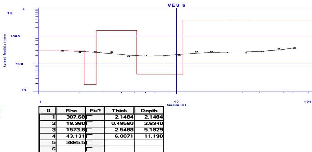
**Figure 3c:** Typical HKH-type curve for 5 layered earth model of the study area northeastern Nigeria.
