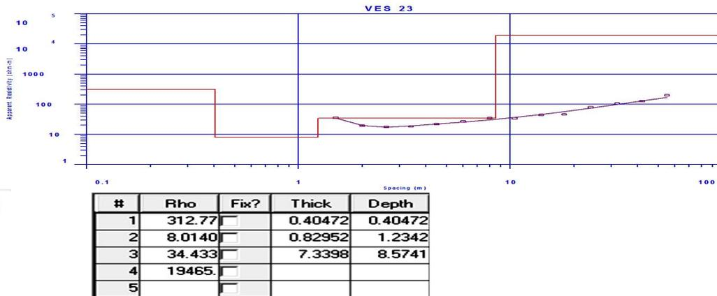
**Figure 3b:** Typical HA-type curve for 4 layered earth model of the study area northeastern Nigeria.
