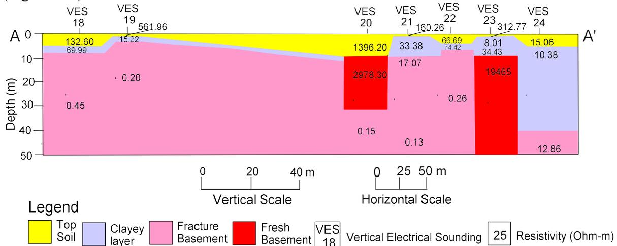
**Figure 11a:** 2-D Geoelectric sections along profile AA’ of the study area northeastern Nigeria.
