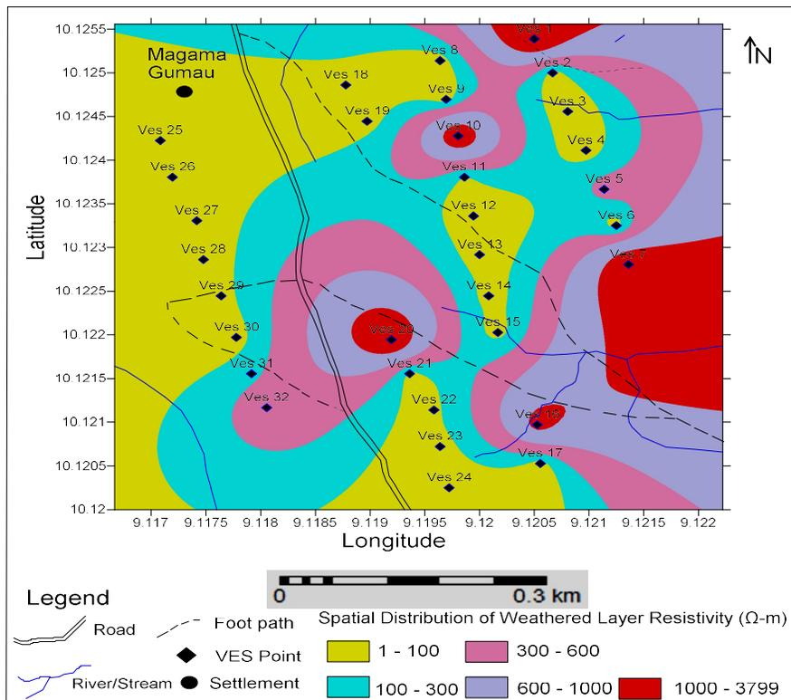
**Figure 6:** Isoresistivity map of the weathered layer of the study area northeastern Nigeria.
