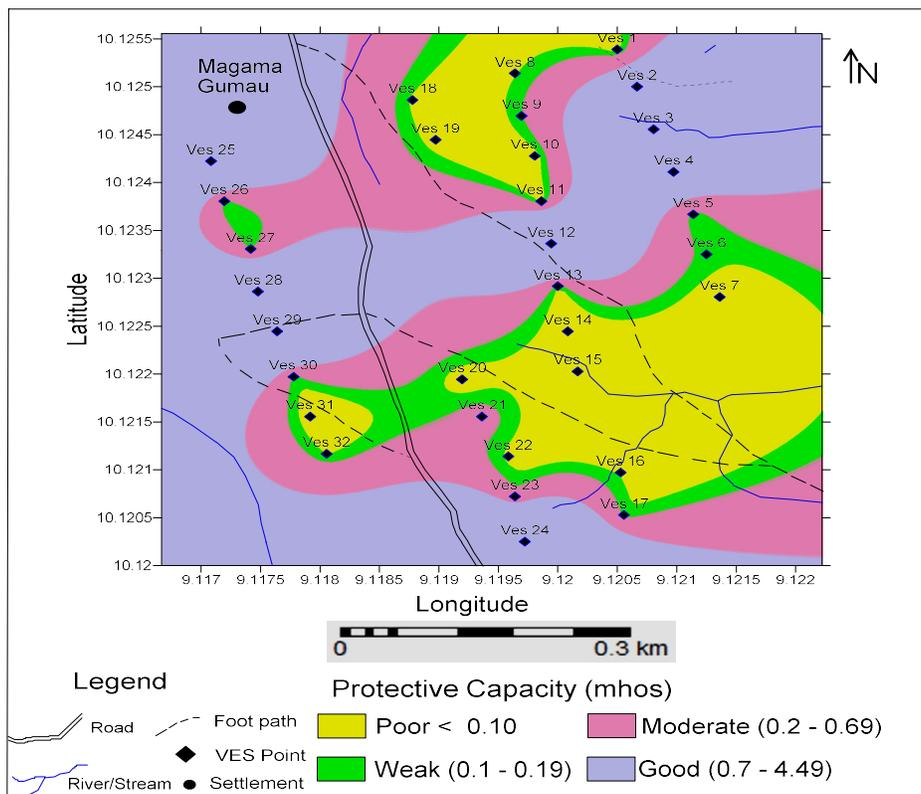
**Figure 8: Overburden protective capacity map of the study area northeastern Nigeria**
