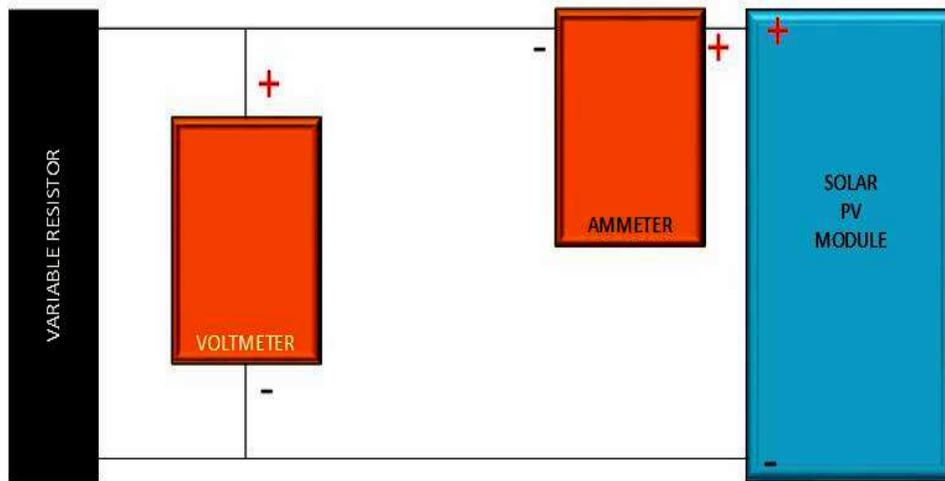
**Figure 3:** schematic experimental set up
