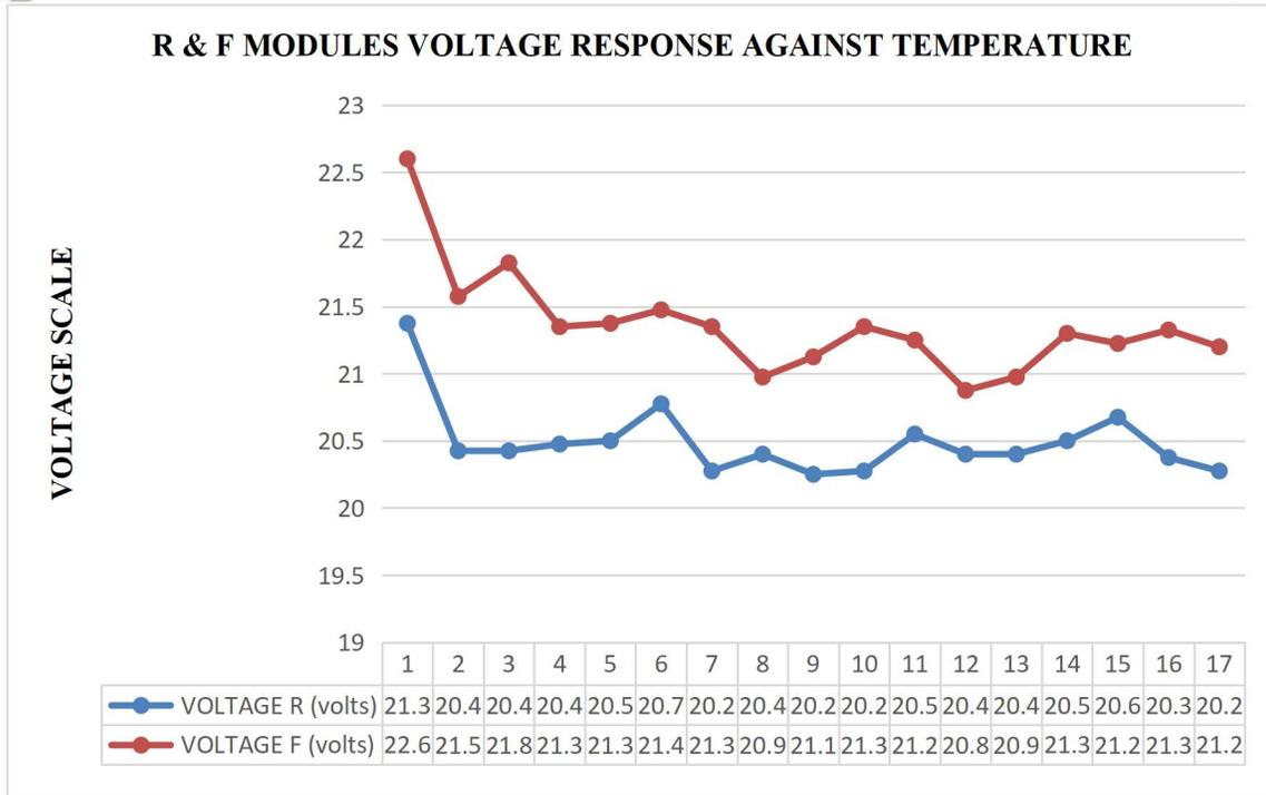
**Figure 6:** Graphical charts displaying temperature voltages fluctuations of both reference and fabricated modules.
