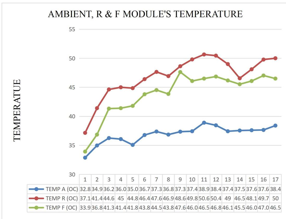
**Figure 5:** Graphical illustration of ambient and modules' (R and F) operational temperatures relationship.
