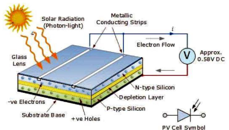
**Figure 1:** A Diagram of a Solar Photovoltaic Cell Showing the Electron-Hole Pairs (Source: Cox, *et al.*, (2020)).
