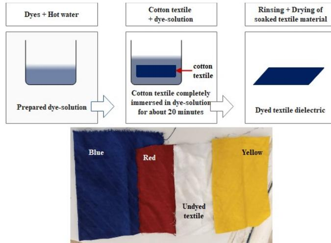
**Figure 1.** Schematic procedures of dyeing cotton fabric and samples of dyed fabrics.
