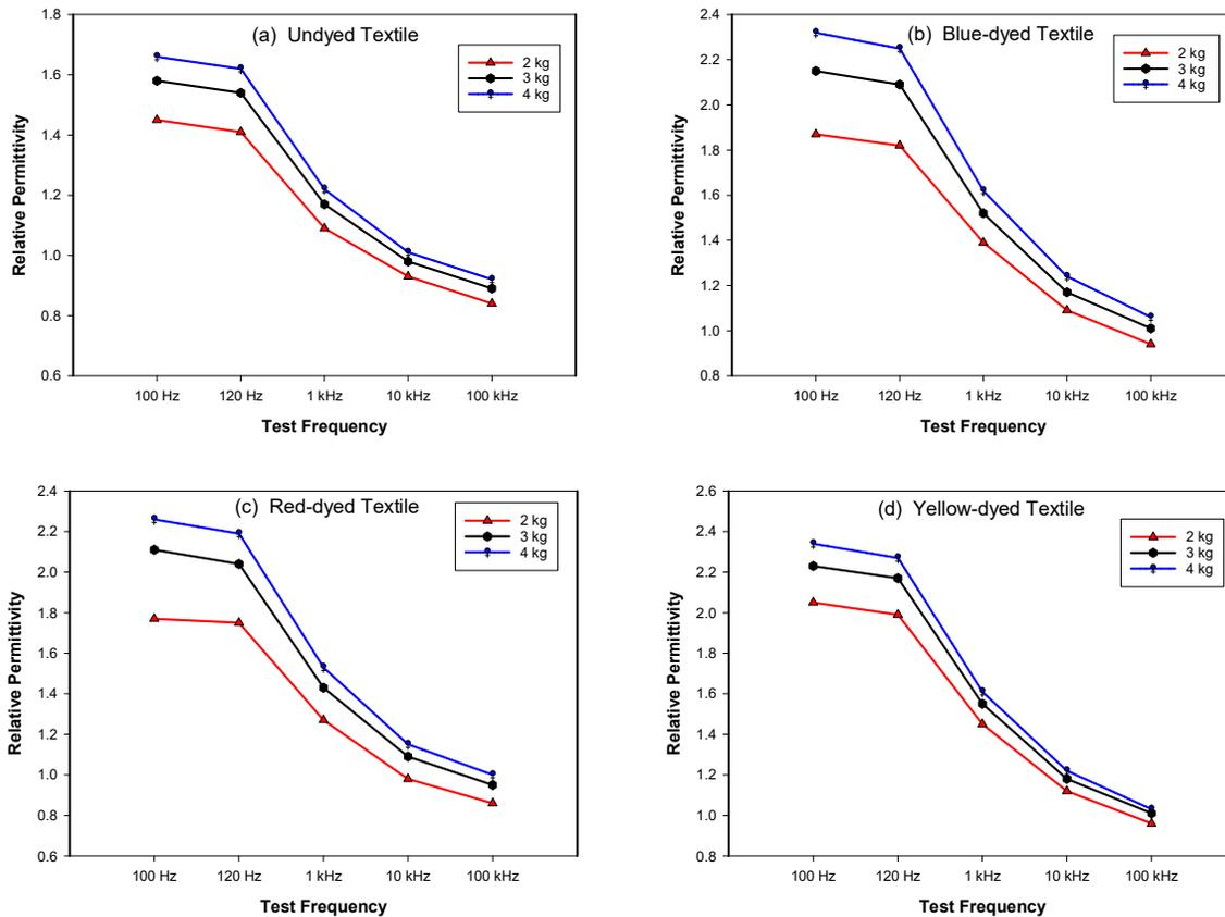
**Figure 3.** Relative permittivity under varying pressure and test frequency for dry (a) undyed, (b) blue-dyed, (c) red-dyed, and (d) yellow-dyed fabric dielectrics.
