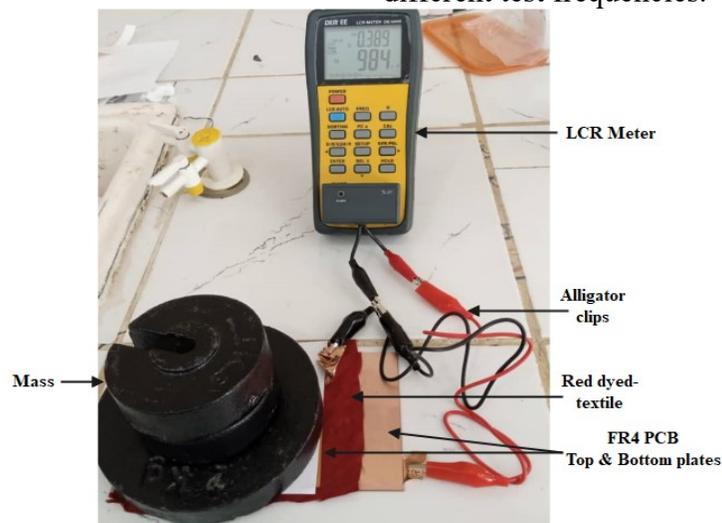
**Figure 2.** Parallel plate method for measuring of capacitance from a red dyed-fabric dielectrics.
