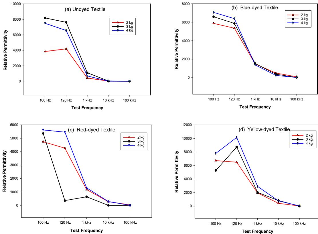
**Figure 4.** Relative permittivity under varying pressure and test frequency for sweat-moisturized (a) undyed, (b) blue-dyed, (c) red-dyed, and (d) yellow-dyed fabric dielectrics.
