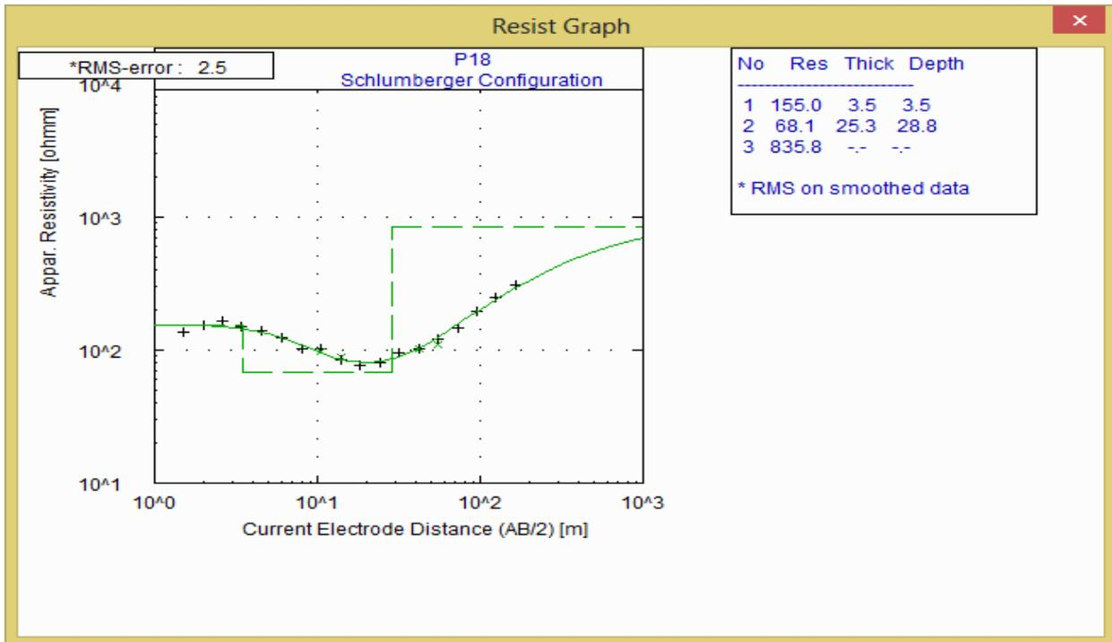
**Figure 3d:** Typical type H curves for 3 layered earth
