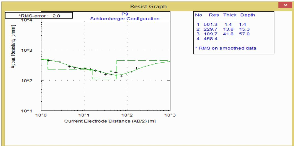
Figure 3b: Typical type QH curves for 4 layered earth
