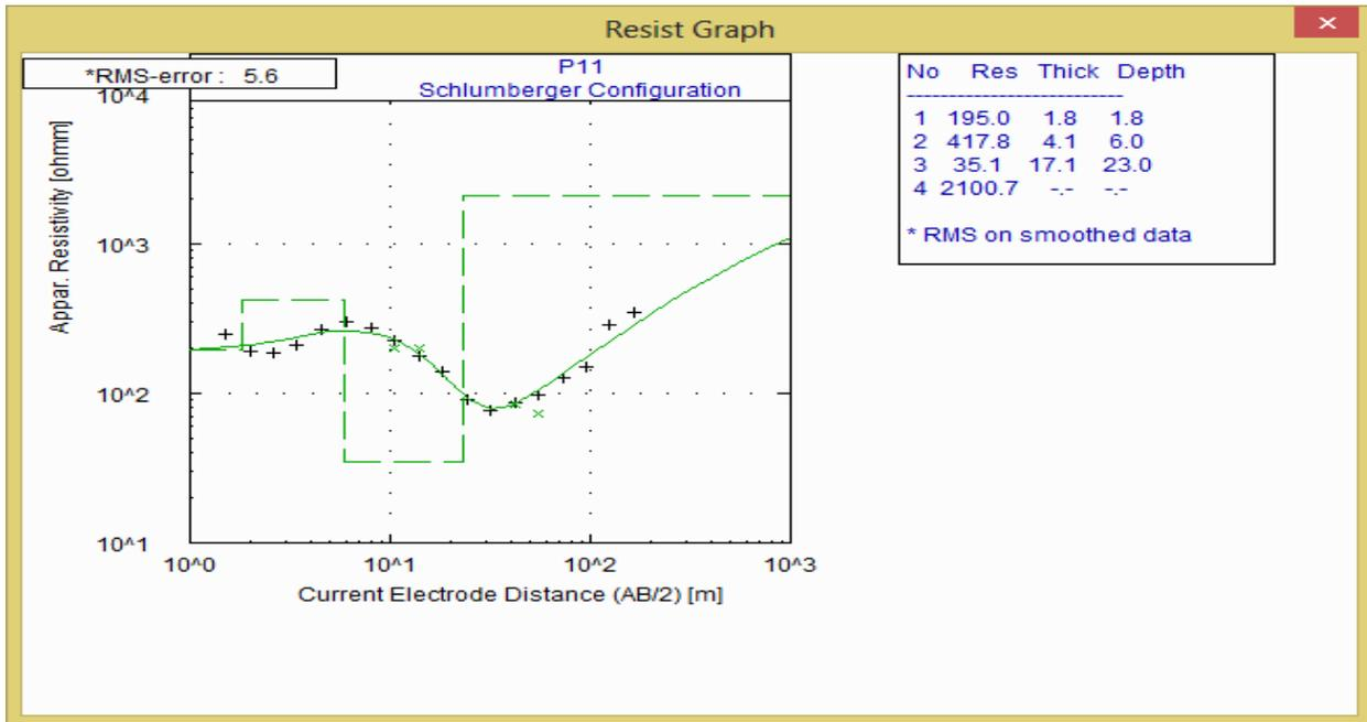
**Figure 3c:** Typical type KH curves for 4 layered earth
