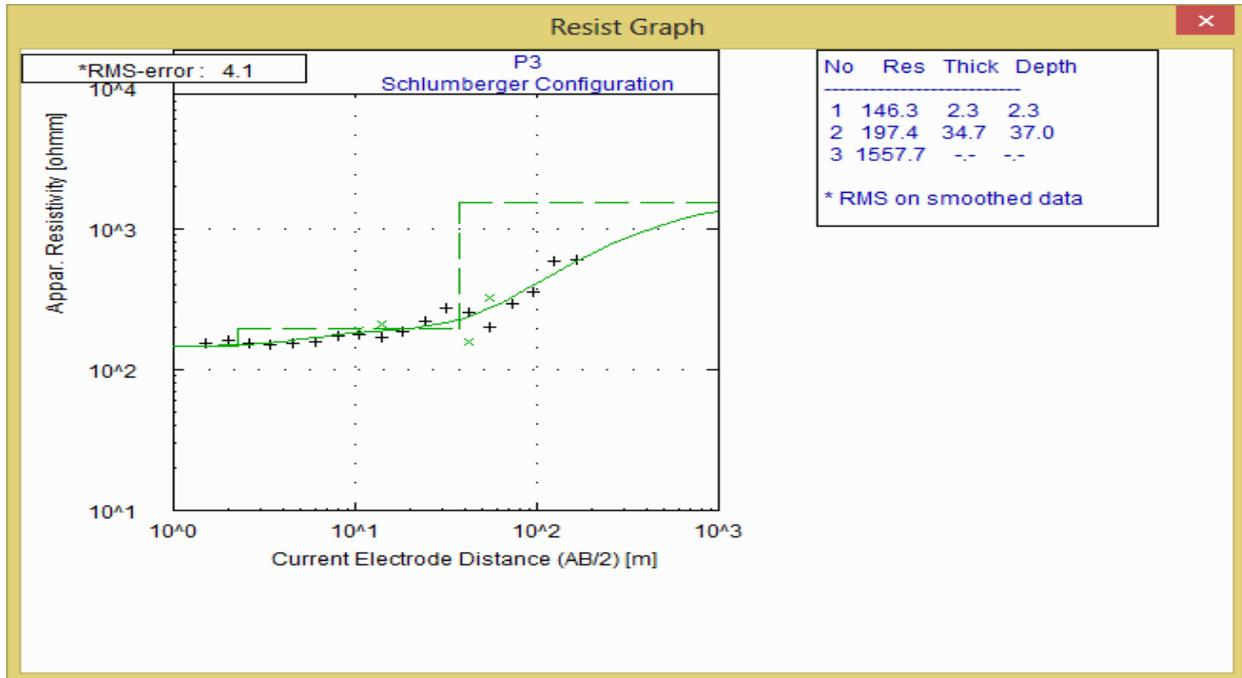
Figure 3a: Typical type of a curve for 3 layered earth
