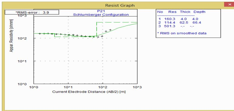
**Figure 3e:** Typical type Q curves for 3 layered earth
