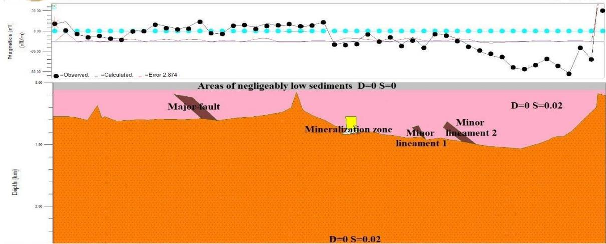
Figure 11: Modeled field of profile BB1, showing calculated and Observed magnetic field readings with depth in km
