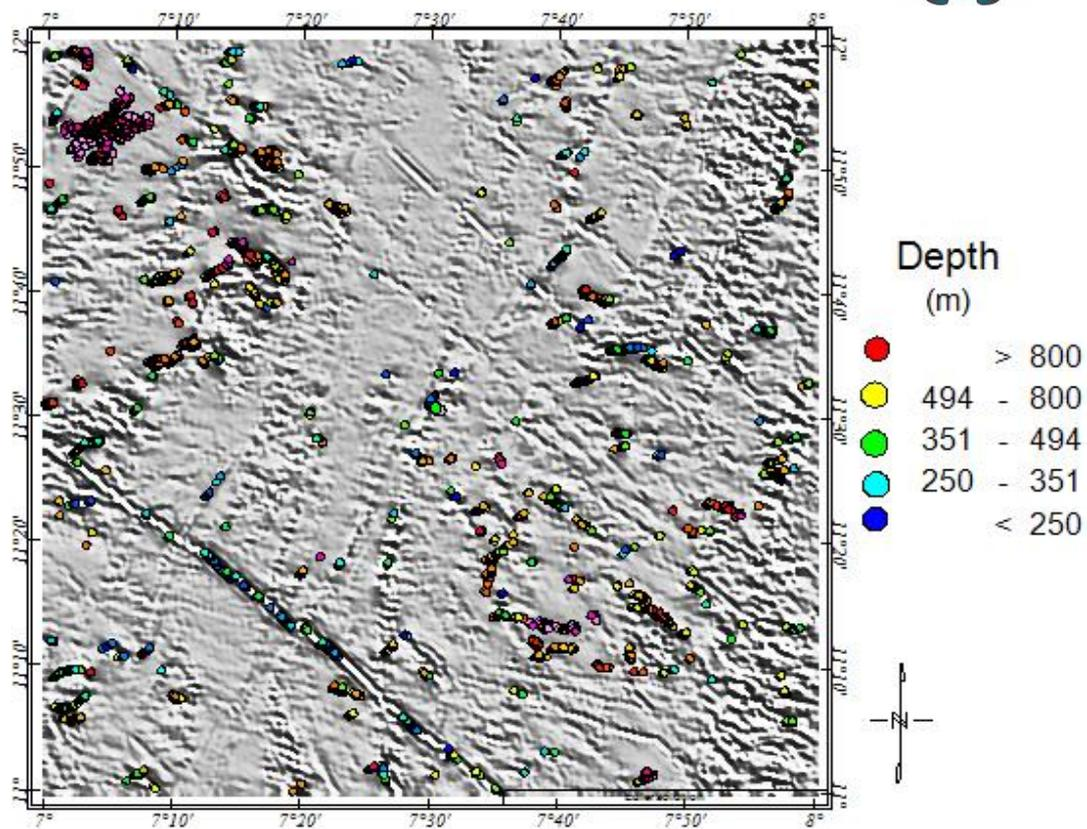
Figure 9: Plot of Euler depth solution.
