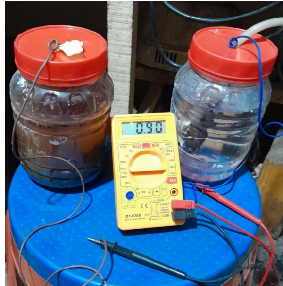
Figure 1: Experimental setup of the microbial fuel cell.
