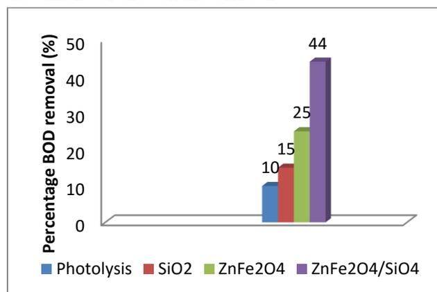
**Fig 5:** BOD removal from textile effluent via photolysis and photocatalysis using  $ZnFe_2O_4$  and 30 wt%  $ZnFe_2O_4/SiO_2$ . [irradiation time – 80 mins. Photocatalyst dose – 0.1 g/L]
