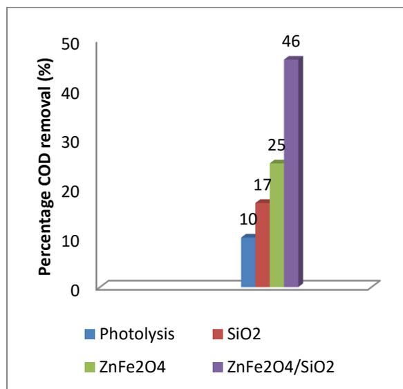
**Fig 4:** COD removal from textile effluent via photolysis and photocatalysis using  $ZnFe_2O_4$  and 30 wt%  $ZnFe_2O_4/SiO_2$ . [irradiation time – 80 mins. Photocatalyst dose – 0.1 g/L]
