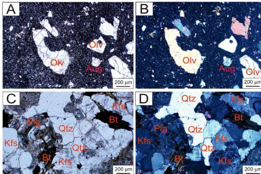
**Figure 5:** Photomicrograph of basalt under PPL (a) and XPL (b) showing phenocryst of olivine and matrix made up of plagioclase laths and iron oxide; photomicrograph of trachyte under PPL (a) and XPL (b) showing zoned plagioclase and flakes of biotite. Plg: Plagioclase, Oliv: Olivine, Aug: Augite, Opq: Opaque; Kfs: K-feldspar
