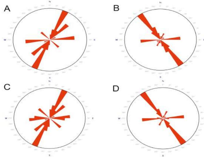
**Figure 7.** Rose Plot for veins (a) and joints (b) for porphyritic biotite granite; rose plot of veins (c) and joints (d) for equigranular granite. Showing NE-SW as the dominant trend for the veins; and NW-SE as the major trend for the joints.
