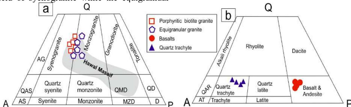
**Figure 8:** (a) IUGS classification of plutonic rocks based upon modal mineralogy After Le Bas and Streckeisen (1991); (b) IUGS classification of volcanic rock based on modal mineralogy (Le Bas and Streckeisen 1991). A = alkali feldspar, P = plagioclase, Q = quartz.
