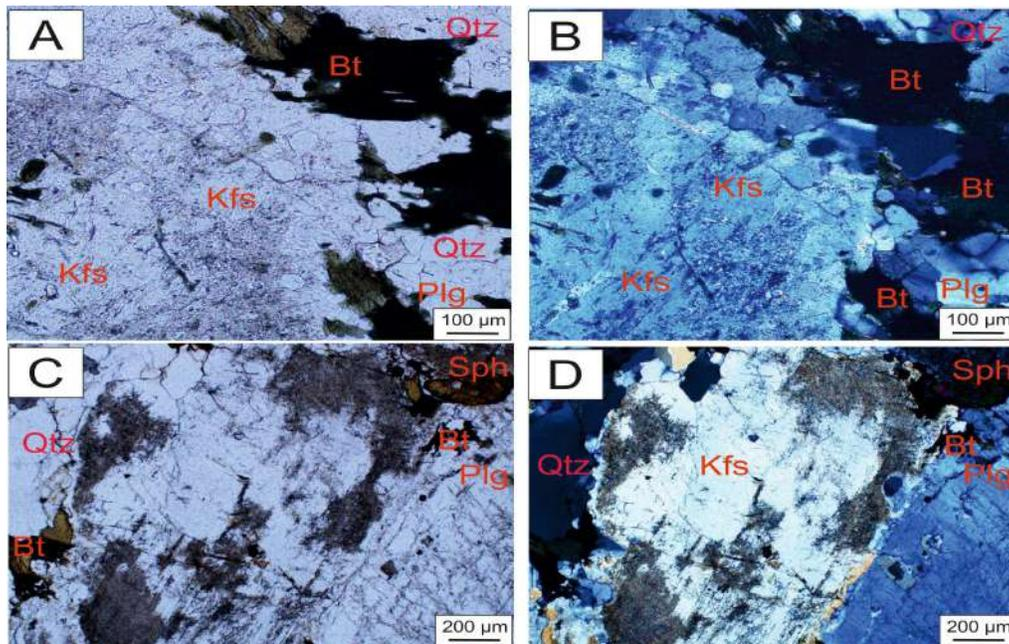
**Figure 4:** Photomicrograph of porphyritic biotite granite under PPL (a) and XPL (b) depicting the phenocryst of microcline; Photomicrograph of equigranular granite under PPL (a) and XPL (b) showing the nearly equal crystal size with sphene (titanite) grains as accessory. Qtz: Quartz; Bt: Biotite; Plg: Plagioclase; Kfs: K-feldspar; Sph: Sphene.
